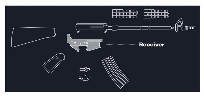
58. Most ghost guns are made from "unfinished" frames and receivers—meaning frames and receivers that are "solid" and lacking in machine marking or drilling in certain specified areas (typically the fire control cavity or trigger area). Unfinished frames and receivers are often
