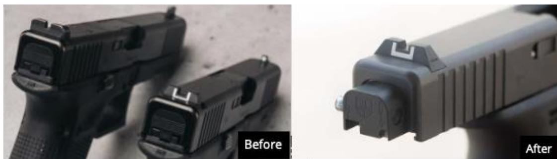
39. The auto sear has a small protrusion called a “disconnecter” that, once installed, pushes the pistol’s internal trigger bar down, allowing the striker to continue firing as the slide reciprocates with recoil. The ability to fire continuously, without the shooter having to pull and release the trigger repeatedly, allows for a much faster rate of fire.
